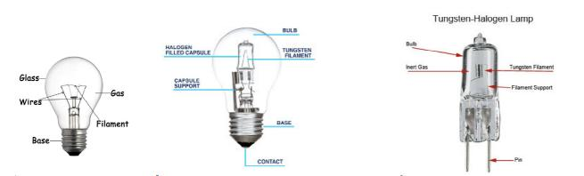
In the classic electric filament bulb a current is passed through a thin, long, metal wire. There resistance to the current creates energy, which is emitted as light (5%) and heat (95%). In a standard bulb, an inert gas is introduced into the glass to reduce combustion of the metal and preserve the life of the bulb. In a halogen bulb, halogen gas is added, making the bulb burn hotter and brighter and reinforcing the filament.
